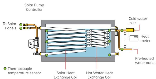
Diagram showing the measurements taken on the Pod
