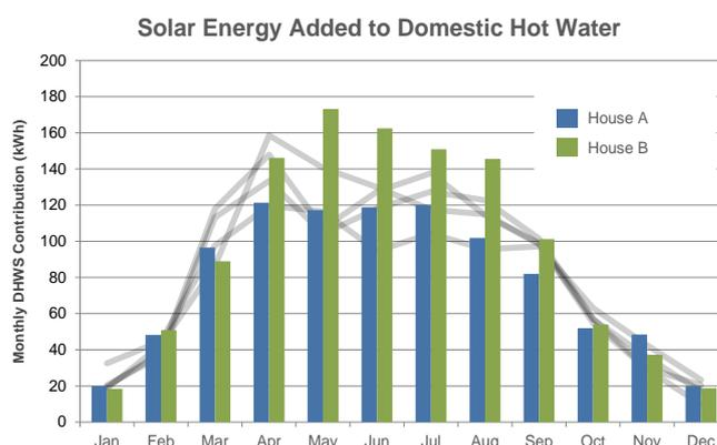
Graph of annual energy output from the Pod compared with a study of four twin coil solar hot water systems (grey lines)
